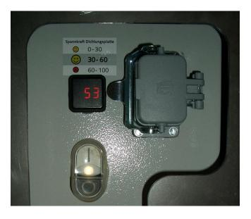
A pictogram is showing the selection of tensioning when the correct tensioning is given.
